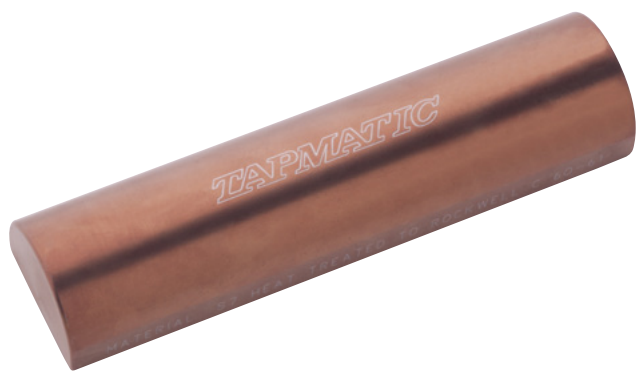
Example marking a curved surface programmed at constant marking plane. Material is S7 tool steel heat treated to 60 HRC. Setting 'H' with 2mm compression at closest point on surface.
