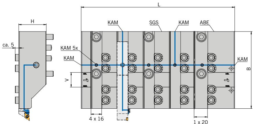
SGS = locking threaded pin – for two separate pressure chambers (high pressure)
