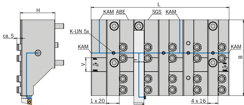
ABE = parting insert rupture detection, Citizen original can be fitted
