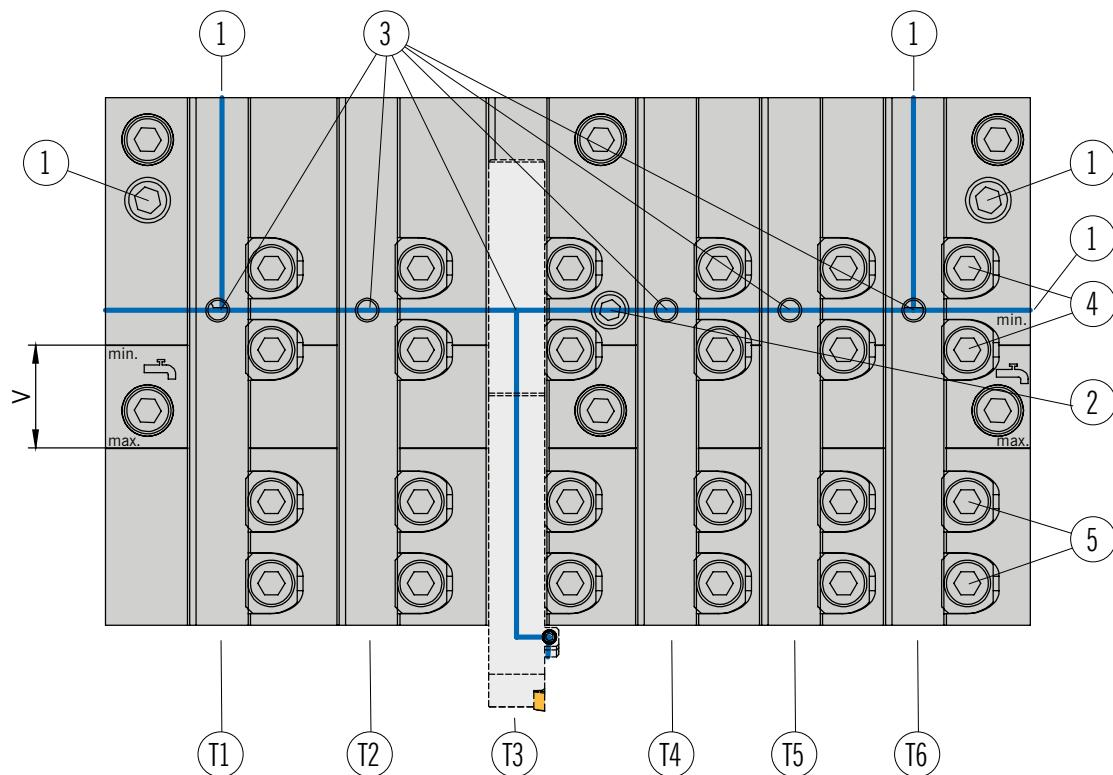
**Tightening torque for clamping wedge AWL-SK111345 = 9 Nm**
